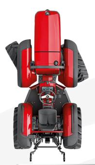
The tractor's **short wheelbase and tight steering radius** provide excellent agility in crop rows. The steering brakes further reduce the turning radius, enhancing the steering effect, which is improved by the doubleacting constant velocity joints.
