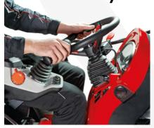
Offers precise proportional control of double-effect hydraulic outlets, lift, and floater, with additional features like continuous delivery activation, hydraulic flow adjustment, PTO on/off, triple position regulation, and Uniflex suspension control.
